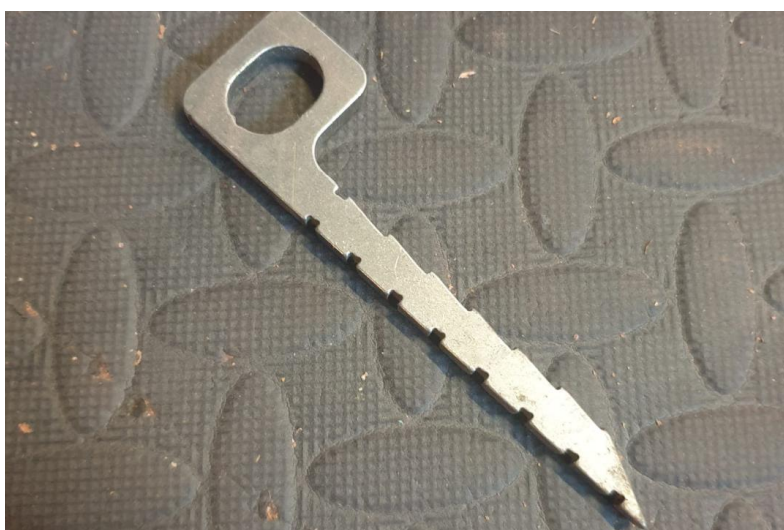
Ecopeg aka pegbolt. Generally drilled and glued into a previous peg placement.
